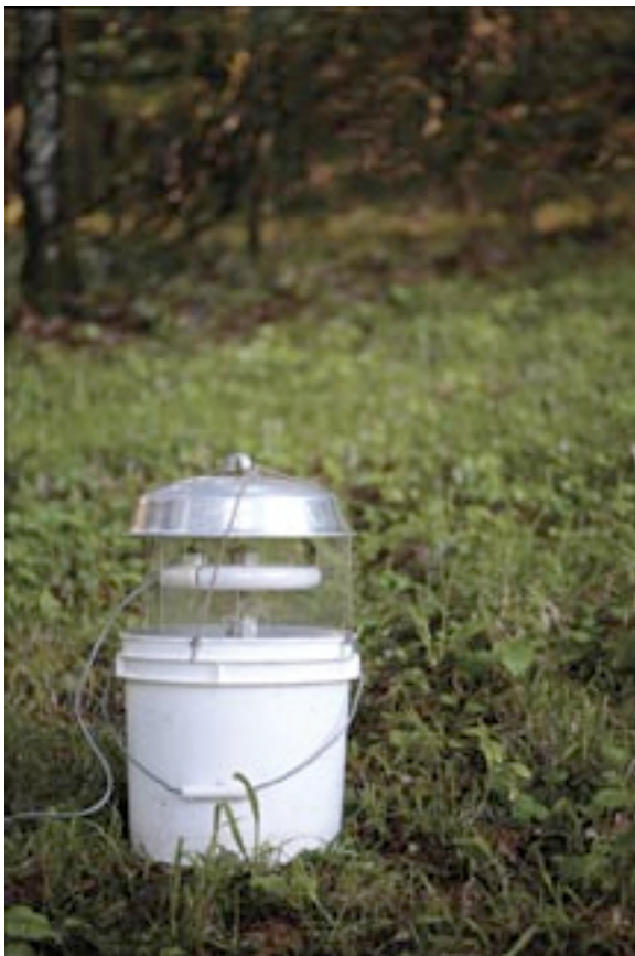
Figure 3-1. Bucket light trap with UV bulb for sampling moths.
